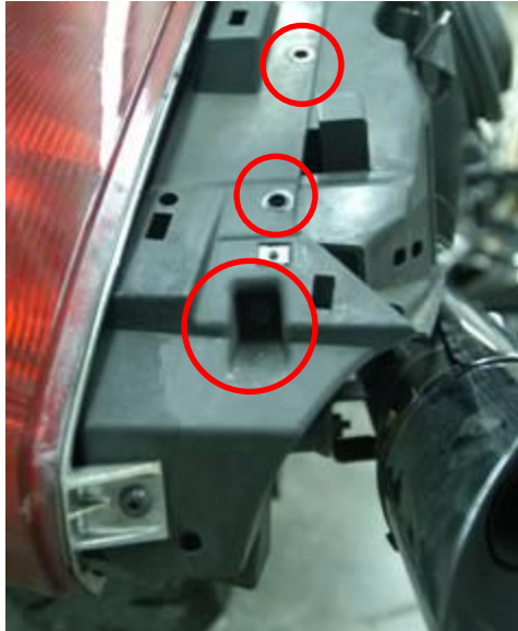
Step 13 & 14-Hex bolt at rear of inner saddlebag in recess. Two holes above are two of the four hex bolts securing inner saddlebag to taillight surround plastic. Remaining two are straight above.
